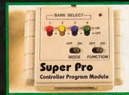
Super Pro Turns any SNES or Genesis controller into a programmable one.
